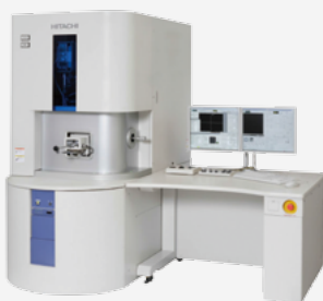
A FIB for Early Analysis of Defects
